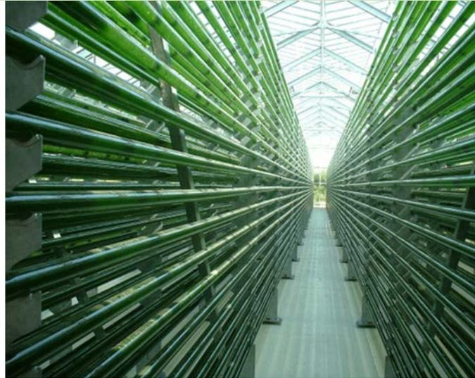
Figure 4: Photobioreactors for algae cultivation in a controlled environment. (Cal Poly).
