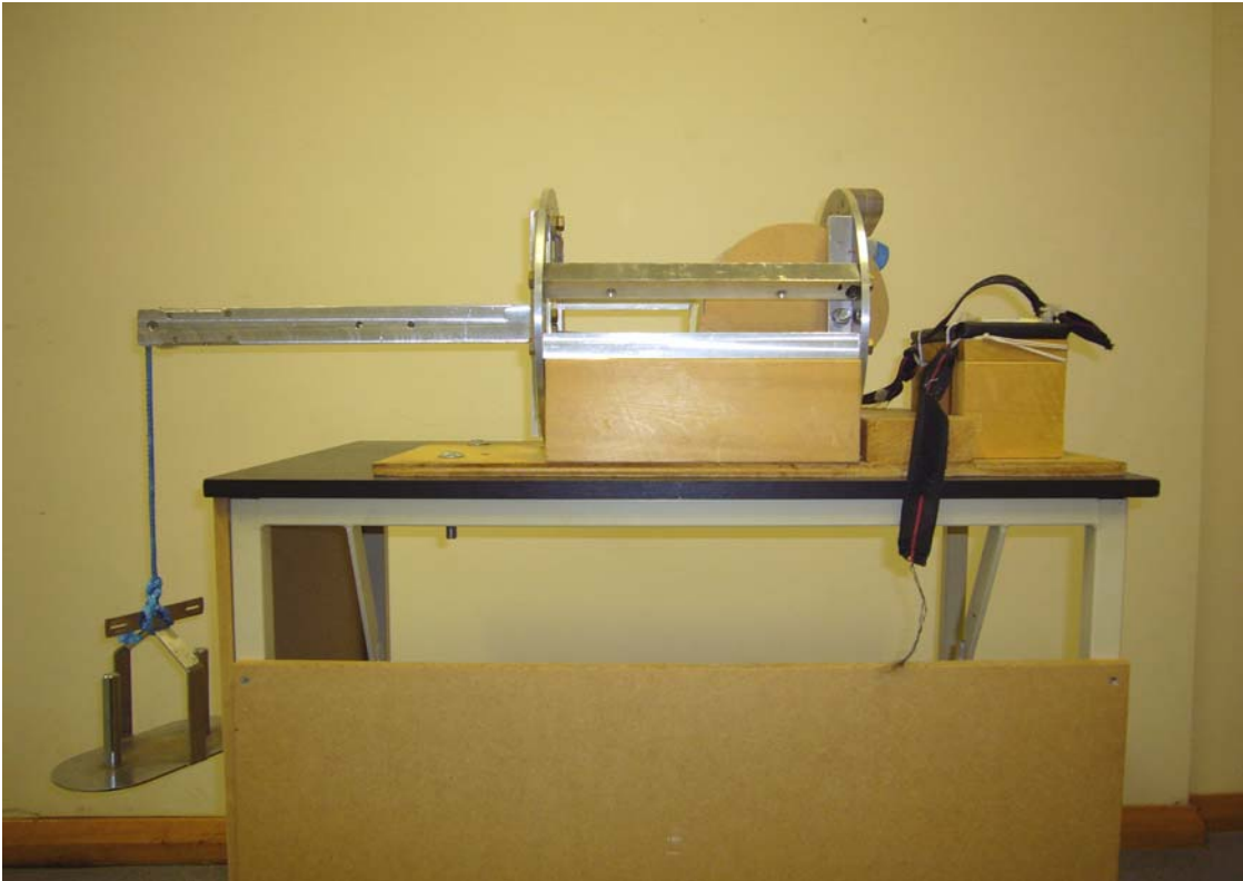
Figure 1: Hand-made arm ergometer used for multiple forearm-wrist flexion.
